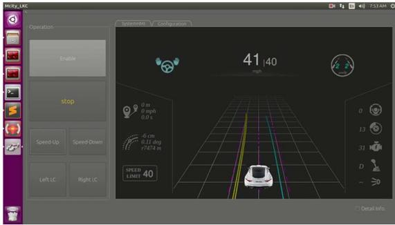
Fig. 20. The software HMI for lane keeping control.
