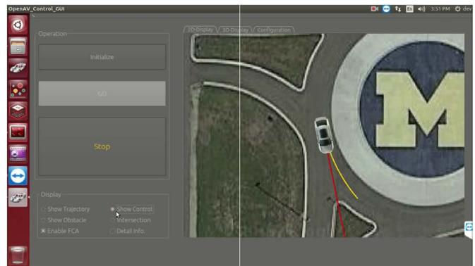
Fig. 7. Developed path-tracking control software HMI.
