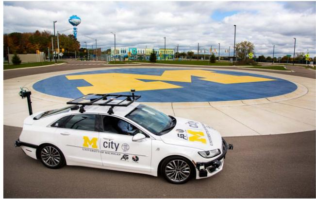
Fig. 6. Automated testing vehicle (a hybrid MKZ) and testing field (Mcity).
