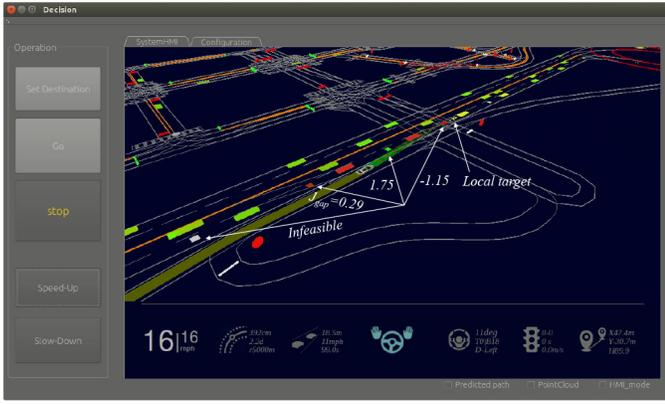
Fig. 19. Interface of our routing and behavior planning software. It shows the gap selection when merging into a highway. The small green square indicates the best gap with the highest score of 1.75, the red squares indicate gap candidates with lower scores, and the gray square indicates an infeasible gap. The yellow triangle indicates the local target.
