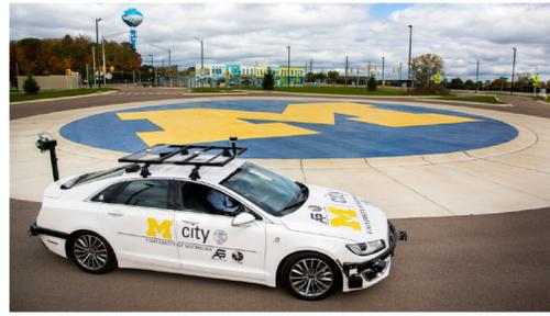
Fig. 21. Mcity automated vehicle platform—a hybrid Lincoln MKZ.
