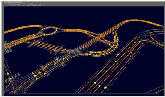
Fig. 2. Developed HD Map of Mcity. The yellow dots are the waypoints and the orange curves are the center lines of lanes or the yellow lane markings.
