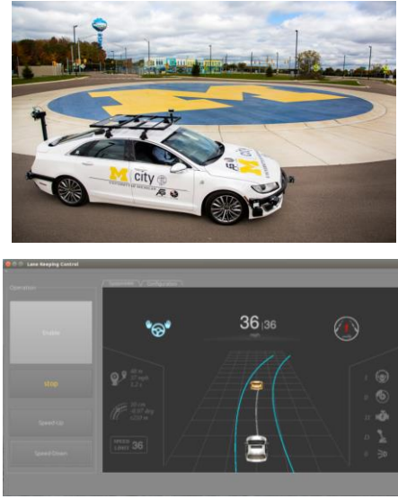
Fig. 5. Automated test vehicle (a hybrid MKZ), testing track (Mcity), and software HMI.
