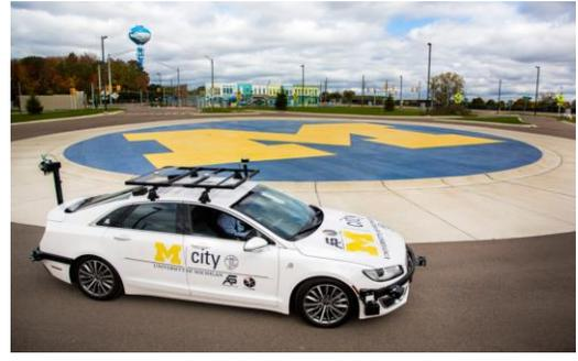
Fig. 3. Automated testing vehicle (a hybrid MKZ) and testing track (Mcity).
